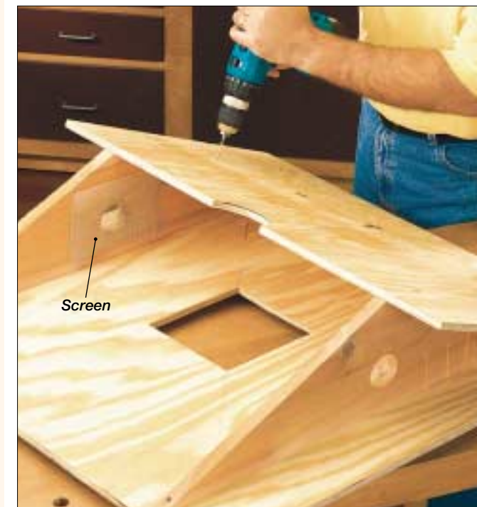
Cover the inside of the gable holes with fine-mesh screen; then assemble the roof components.
